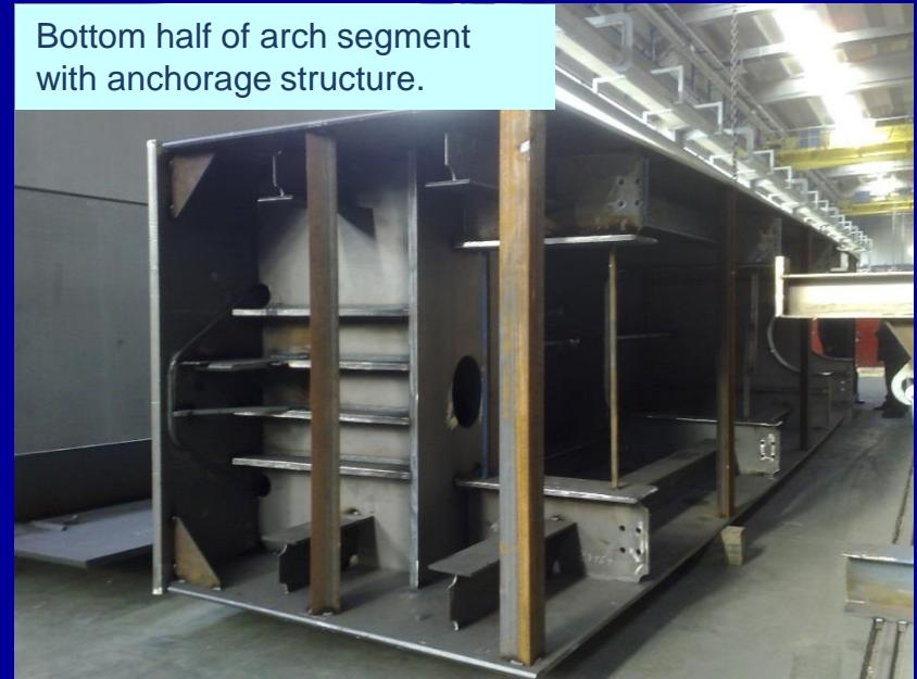
Bottom half of arch segment with anchorage structure.
